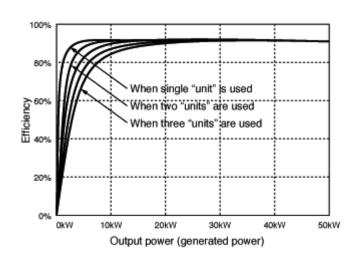
Fig.5 Running efficiency of 50kW "PMB"
