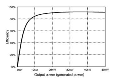
Fig.4 Running efficiency of the conventional model
